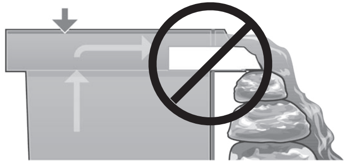
Fig. 17 If a thick rock along with a larger flow pump is used, the water flow may be so great that it will flow over the sides of the BIOFALLS® filter.
